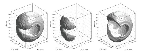
Figure 2. The *reachable space* of the Nao's hand is approximated by a three dimensional grid; (left) the theoretical reachable grid generated in simulation; (right) reachable positions with the fixed yaw-joint in the elbow; (center) difference between both grids;
